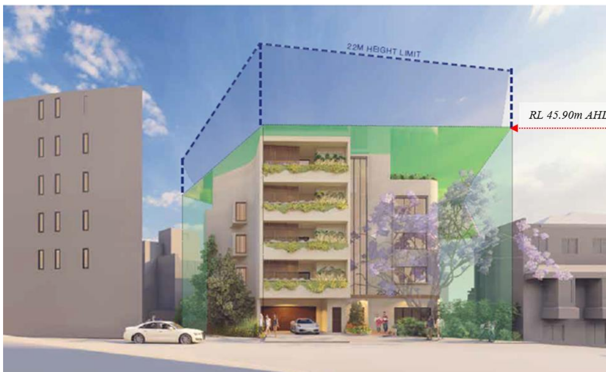
Figure 5: Proposed building envelope: maximum 22m height envelope shown with dashed line and secondary height plane of RL 45.90m AHD shown in green (Source: Antoniades Architects)
