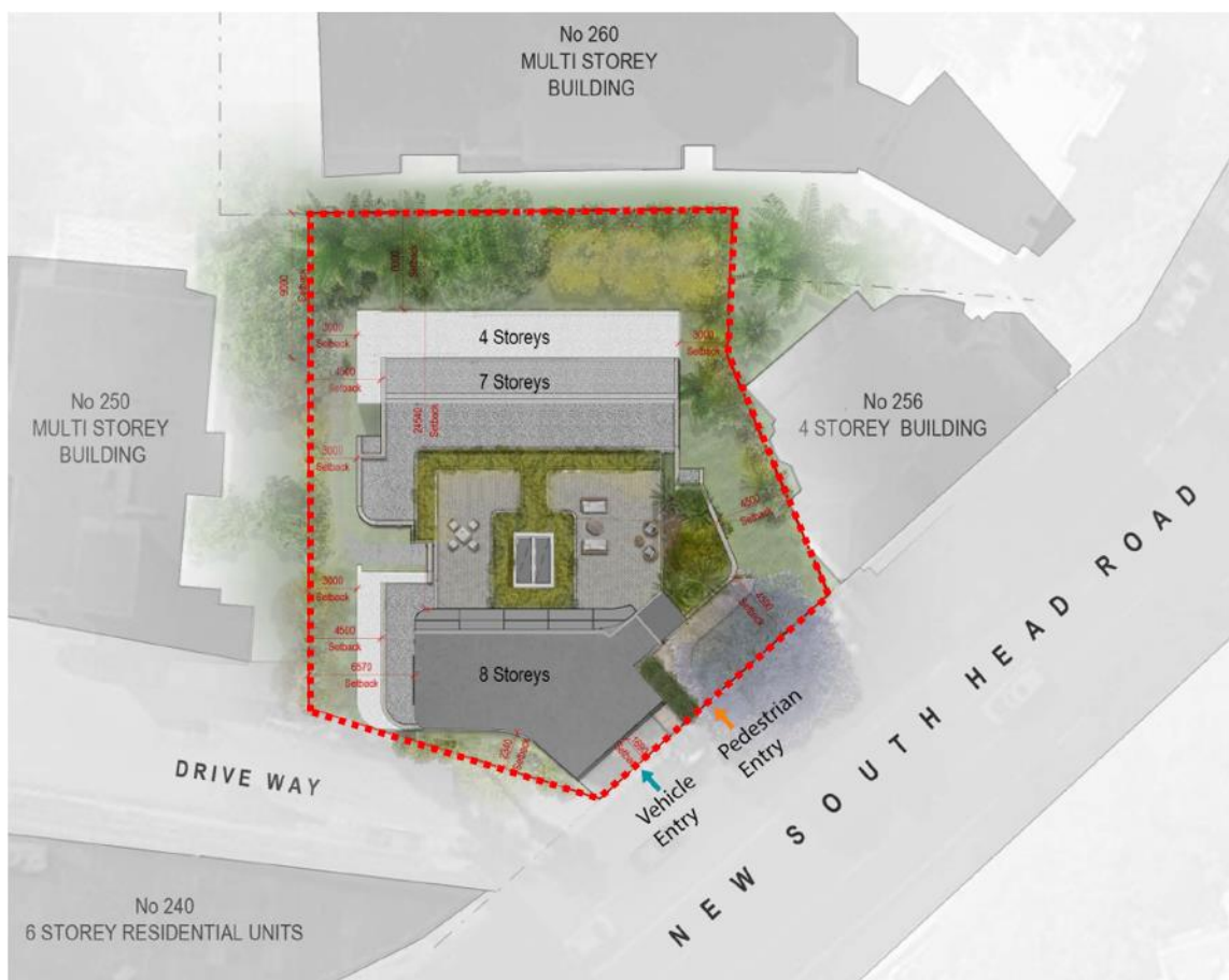
Figure 7: Indicative development concept site plan: illustrating the proximity of the development concept to the site boundary and the neighbouring buildings. (source: Antoniades Architects).
